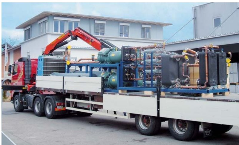
Depending on the installation conditions, KWT heat pumps can be delivered as modules.
